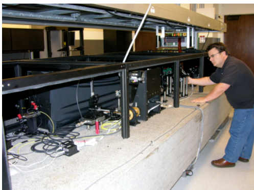
Figure 2. Top: ExAO testbed layouts, from MEMS testing interferometer (Phase 1) to planet imager instrument prototype with diffraction-suppressing coronagraph (Phase 2). Bottom: Left: lab engineer Daren Dillon adjusts the alignment of optics on the testbed. Right: a visitor views a MEMS device through a magnifier.
