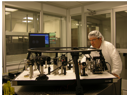
Lab Engineer Daren Dillon assembles the Villages adaptive optics system in the LAO cleanroom facility.
