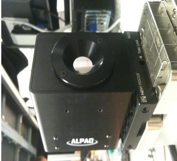
Figure 3. Woofer DM: ALPAO 52-actuator magnetically actuated membrane deformable mirror.
