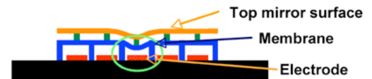
MEMS electrostatic actuator concept (Tom Bifano, BMC)
