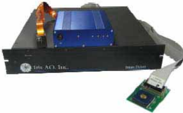
Figure 4.14: Second generation drive electronics with and flex-circuit mirror interface board (upper small box and narrow flex cable) atop the first generation electronics and mirror interface board. Second generation electronics with USB computer interface will be available July 2007.
