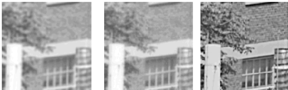
Figure 4.10: Left frame: Conventional image taken with uniform illumination. Center frame: Reconstructed composite with f_o = 0.5 f_c , SNR of 100, using estimates of the phase shift. Right frame: Reconstructed image with f_o = 0.91 f_c , no noise, using estimates of the phase shift.
