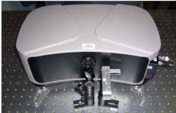
Figure 4.13: AO-equipped Zywave aberrometer modified by Iris AO. Iris AO managed to add AO capabilities within the footprint of the clinical device.
