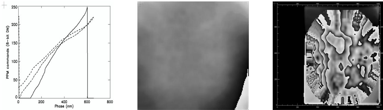
(a) Plots of PPM response curves, 8-bit PPM commands vs. real phase in nm, for several PPM pixels.
