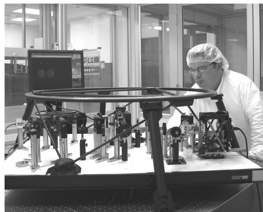
Figure 5. Optical assembly under test. A display of the Hartmann dots from a test beam shows on the monitor.
