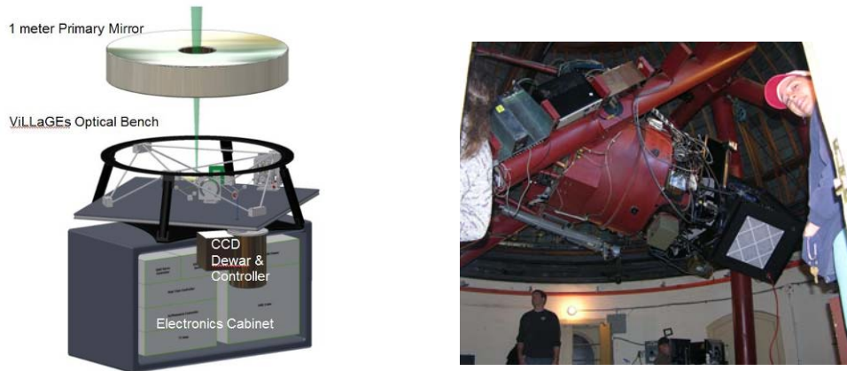
Figure 1. The Villages Adaptive Optics breadboard is attached to the Cassegrain mounting position of the Nickel Telescope. The electronics cabinet houses readout electronics for the wavefront sensor, the wavefront reconstruction computer, and the drive electronics for the MEMS deformable mirror.
