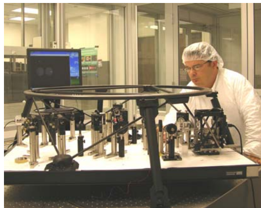
Figure 4. Optical assembly under test. A display of the Hartmann dots from a test beam shows on the monitor.
