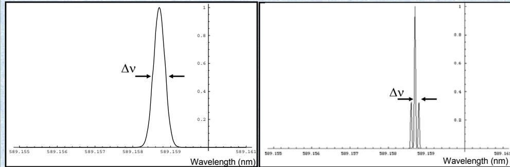
Example of a broad linewidth source or a narrow source with a frequency jitter
