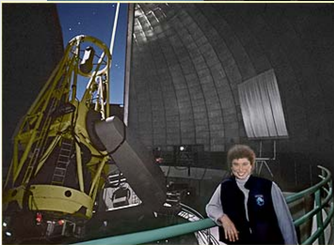
Claire Max stands next to the Shane Telescope at Lick Observatory on Mt. Hamilton. In the background, the bright straight line at the top of the photo is the laser beam from the laser guide star system Max designed as part of the telescope's adaptive optics system, which corrects for the blurring effect of the atmosphere. Photo by Laurie Hatch, Lick Observatory
