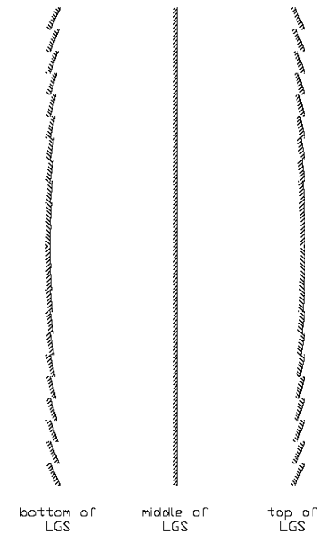
Figure 4- 8: Shape of segmented MEMS during tracking of a LGS pulse. Amplitudes are exaggerated.
