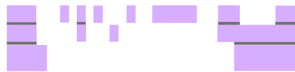
(g) Backside patterning and DRIE followed by directional oxide etch from back and front-side (Mask 4)
