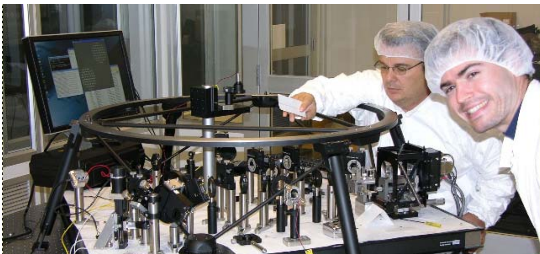
Figure 11. Lab engineer Daren Dillon and graduate student Mark Ammons perform final alignments on the Villages instrument in the LAO. Hartmann sensor readout is shown on the display behind them.
