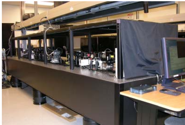
Figure 1. MCAO/MOAO Testbed showing major element and highlighting its reconfigurability for multiple guidestar wavefront sensors, closed loop (MCAO), and open loop (MOAO) architectures
