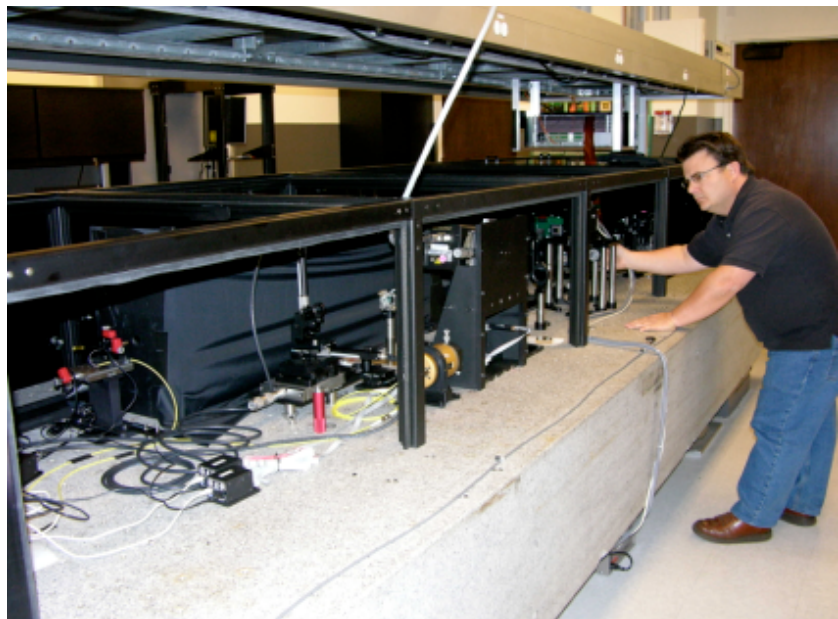
Figure 2. ExAO testbed progress from MEMS testing interferometer (Phase 1) to planet imager instrument prototype with diffraction-suppressing coronagraph (Phase 2).
