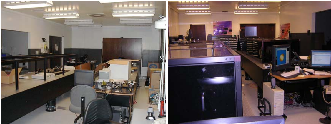
Figure 1. Moving in to the Phase 1 facility in Room 191 of Thimann Laboratories. Left: (April 2004) the two honeycomb steel optical tables, with a light enclosure under construction on one table and various optical components being set up. Right: (July 2004) the ExAO experiment's PSDI interferometer within its enclosure on the left table and MCAO testbed area on the right. The MCAO table contains the Quadrature Polarization Interferometer for qualifying and characterizing the spatial light modulators and a general-purpose commercial Fizeau interferometer for optical measurement of MEMS devices and other optical components.
