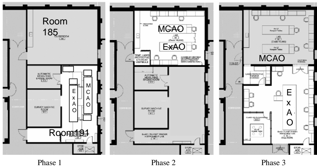
Figure 2. Laboratory for Adaptive Optics Facility Plan. Phase 1, partial refurbishment of Room 191 (completed in March 2004). The ExAO and MCAO experiments now share this space on two honeycomb steel optical tables. Phase 2, refurbishment of Room 185, scheduled to be complete in October 2004, at which time both experiments will be moved there. At the completion of Phase 3, in February 2005, MCAO will inherit the two steel optical tables and the ExAO testbed will move to Room 191 onto a granite optical table. Phase 1 is interim, with only moderate temperature and lighting control. Phases 2 and 3 will have precise temperature, lighting, humidity, and dust control.
