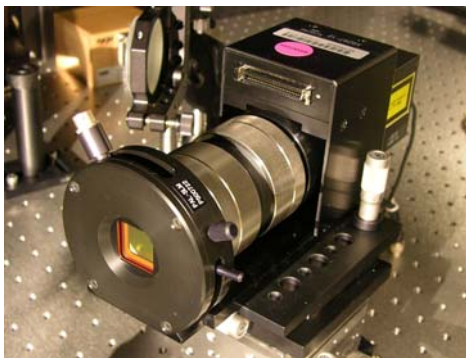
Figure 9. This liquid crystal spatial light modulator (SLM) acts like a deformable mirror with the polarized laser light used on the MCAO testbed. Its 768x768 pixelated array can be used to emulate any of the candidate astronomy deformable mirrors
