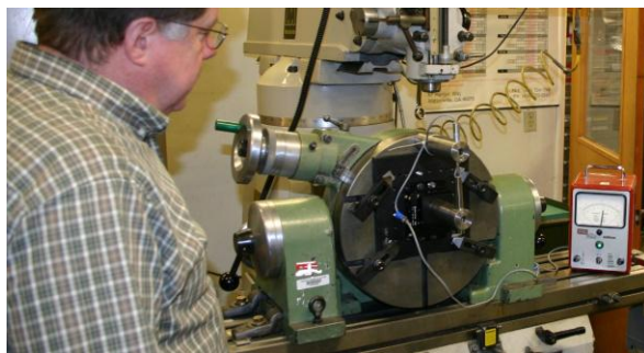
Figure 3. Precision laboratory testing of the deflection of a prototype mount design.
