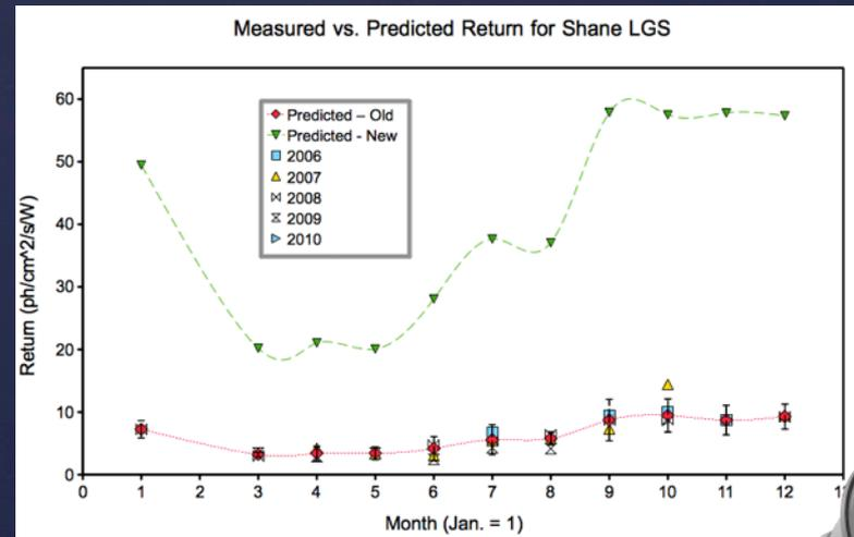
Predicted return of new laser: 5 – 10 x the of the current dye laser at Lick
