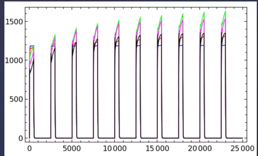
Pulse format of fiber laser (400 ns, 500 kHz, 20% duty cycle) shows inter-pulse optical pumping
