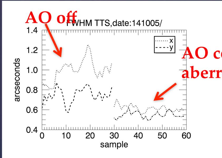
AO correcting static aberration
