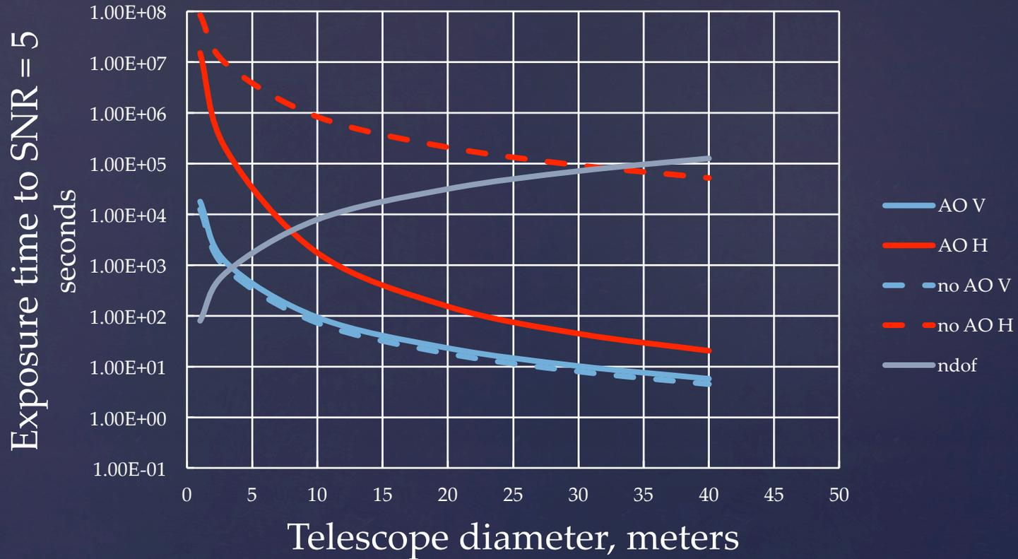
Exposure time to a given SNR as a function of telescope diameter and science band, with and without AO. "Signal" is counted in the diffraction-limited core (AO case) or seeing disk (no AO case). Noise is a combination of background, thermal emission, dark current and read noise, with backgrounds and emission counted only in the pixel region of the signal photons. Assumptions are  $r_0$  = actuator spacing = 10 cm, warm fore-optics, throughput = 50%.
